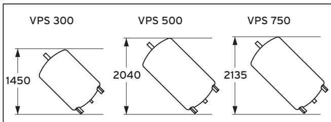
Fig. 4.6 Tilt measurement
