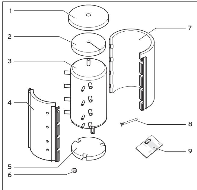
Fig. 4.1 Scope of delivery
