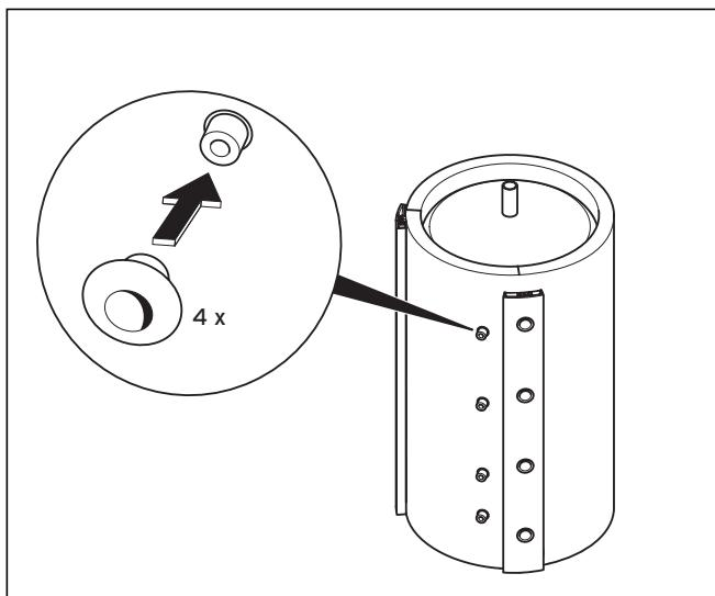
**Fig. 4.12 Attaching the rosettes**
