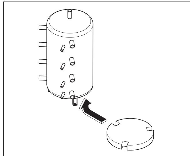
Fig. 4.7 Fitting the bottom pad
