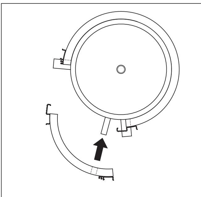
**Fig. 4.9 Attaching the rear insulating jacket (from above)**
