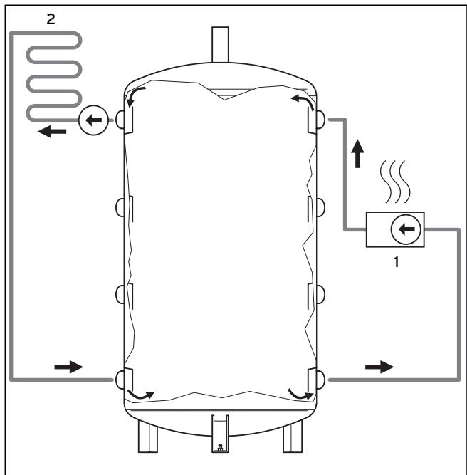
Fig. 2.1 Principle of operation of the buffer cylinder
